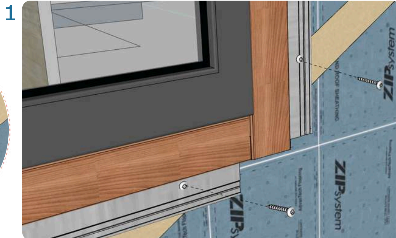
Hard fastening the LUXYCLAD® 1" precision J-Trims with #8 Pan Head Screws.
