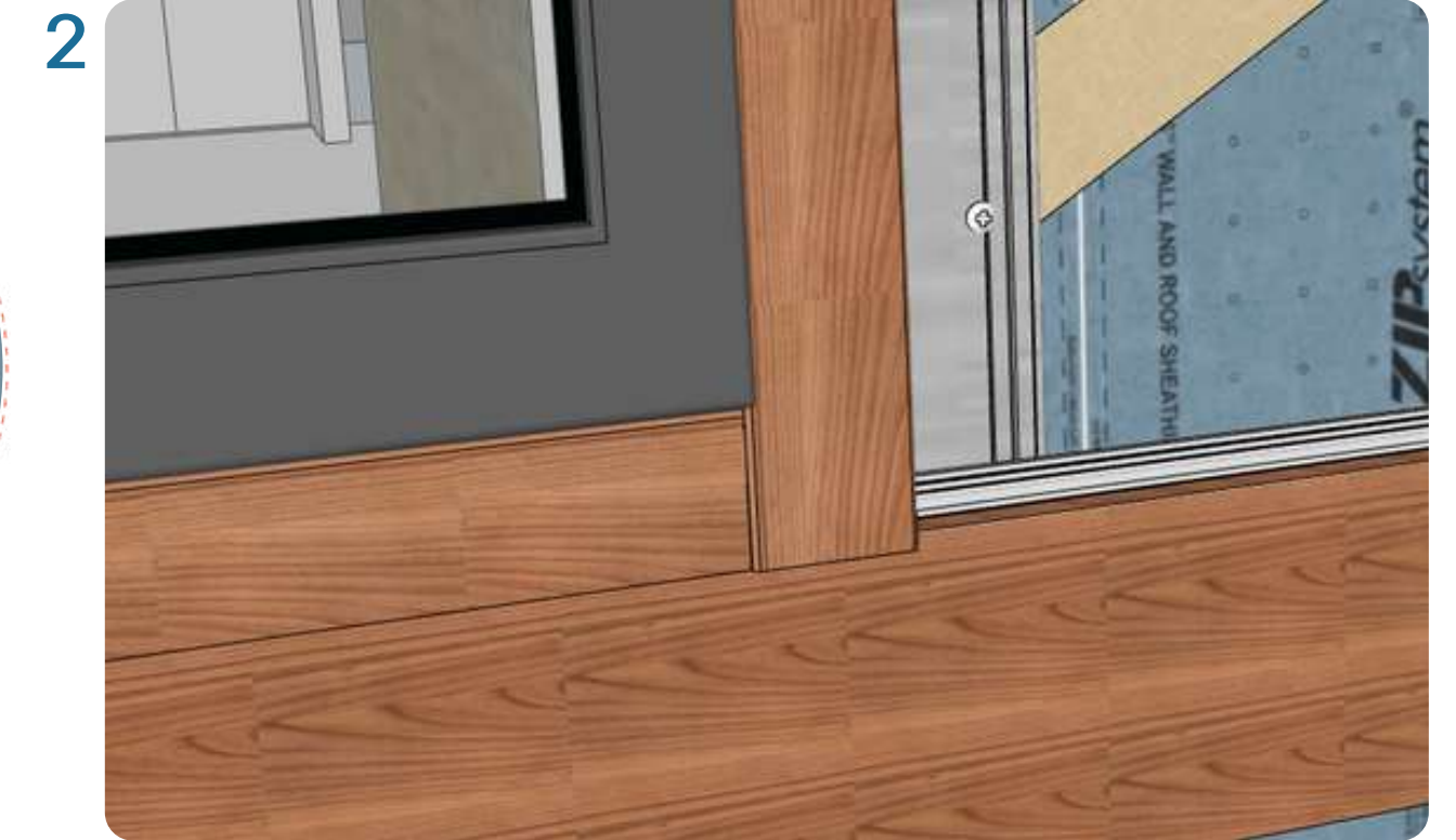
Note: Top support of first siding board must be cut to rest inside the 1" precision J-trim.
